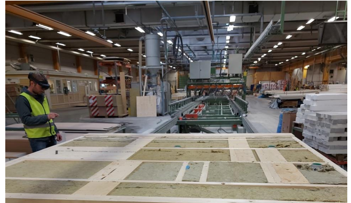
Fig.5 Quality inspection of a timber frame element using HoloLens2
